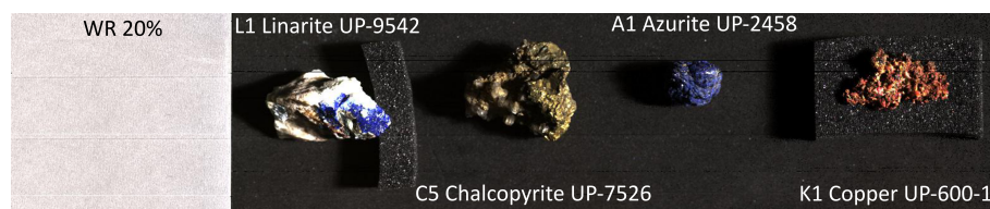
Figure 4. Showing HySpex scan MH_FK_LAB_Cudetect_008_09012018_WR20 as an example to highlight the lack of sample preparation.
