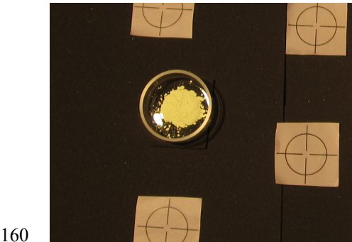
160 Figure 2: Holmium-oxide powder in the laboratory HySpex setting in a quartz glass petri dish underlain by black cellular rubber. Geometric markers for the pre-processing were placed alongside the sample.
