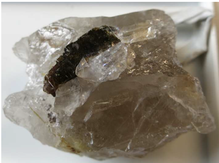
165 Figure 3: Xenotime embedded in quartz as an example for the REE-bearing mineral samples.
